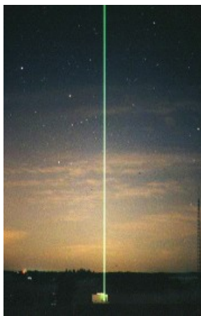
Figure 1 In this photo taken by Luc Girard, the University of Western Ontario's Purple Crow lidar sends laser light into the atmosphere. The laser light reflects off air molecules, revealing information about the atmosphere.
