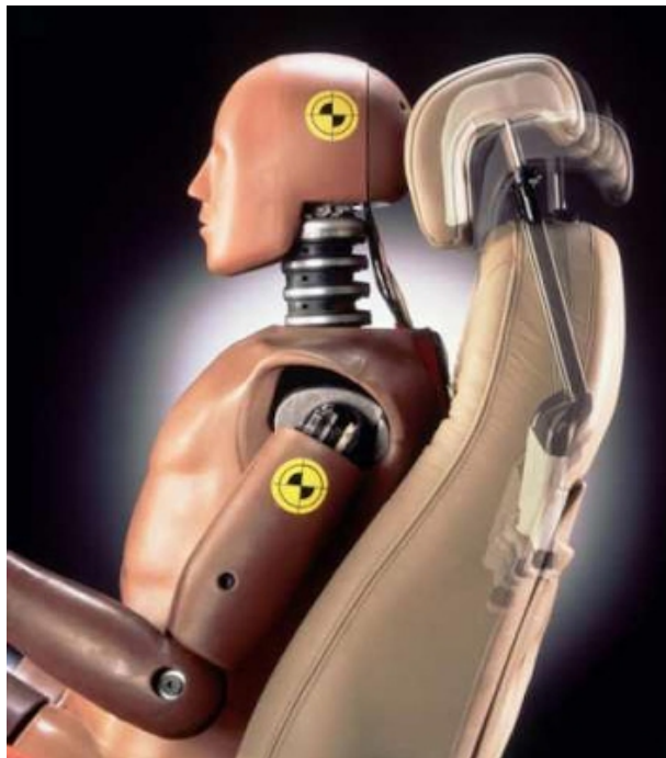
Figure 1 Active head restraints protect a passenger's head and neck during low-impact rear-end collisions.
